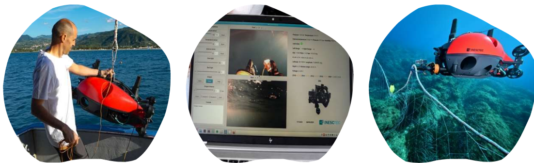
Figure 16. IRIS robotic system being deployed (left), computer interface (middle), and approaching a tagged fishing net (right).
