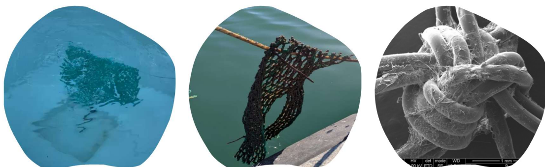
Figure 20. Picture of the net submerged in the mesocosms experiments (left) and in situ experiments at Póvoa de Varzim fishing harbour (middle); fishing net surface after immersion in seawater under environmental conditions (right).
