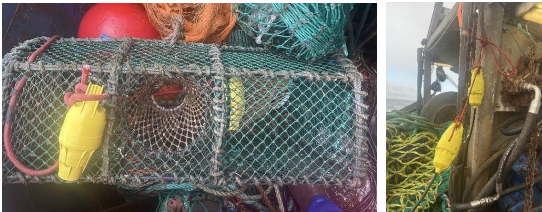
Figure 20 - Tags attached to prawn creel (left) and SLUs at stern of vessel (right)
