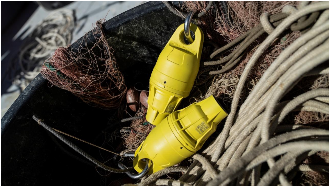
Figure 3 - MGT transponders (tags) attached to trammel net (Photo credits: Claudia Amico)
