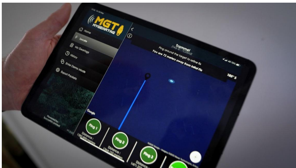
Figure 6 - MGT app guiding the vessel towards the estimated tag position (Photo credits: Claudia Amico)
