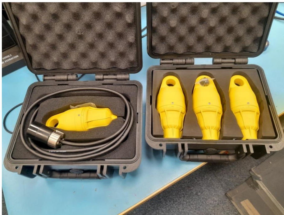
Figure 2. Production NETTAG+ SLU (left) with production tags (right).
