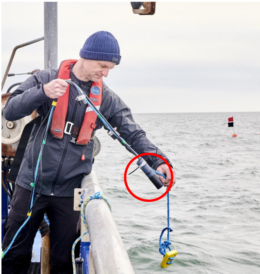
Figure 5. Directional SLU transducer element deployed alongside standard omnidirectional SLU.
