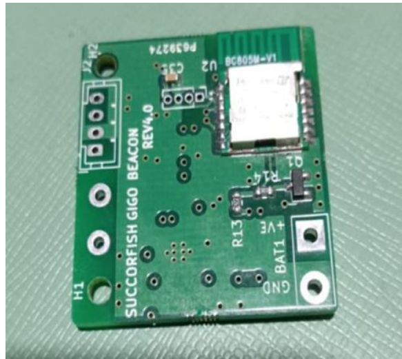
Figure 4. Bluetooth wireless interface board used in production wireless SLU.
