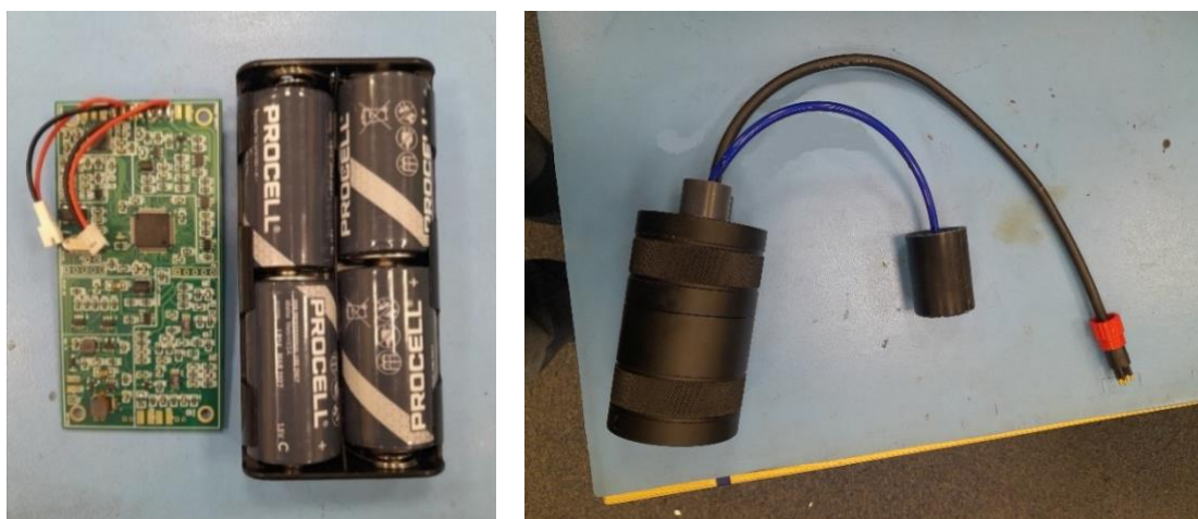
Figure 11. NanoPAM Live demonstration unit: (left) circuit and battery, (right) waterproof housing containing circuit and battery with receiving hydrophone and connector to radio antenna.
