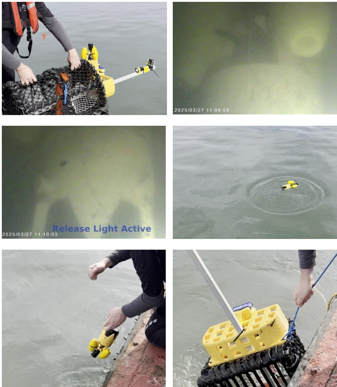
Figure 3. (top left) Deployment of system on lobster trap (note: protruding pole added to hold camera for underwater footage and not part of system), (top right) underwater view of release unit on seabed, (middle left) release unit activated, (middle right) arrival on surface, (bottom left) retrieval of thin release line, (bottom right) recovery of trap via equipment line.
