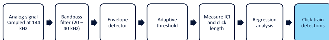
Figure 6. Signal processing steps for dolphin click detection algorithm.
