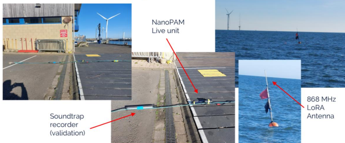
Figure 12. Deployment of prototype click detector system from surface buoy with radio transmitter.
